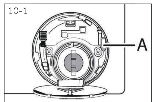
When the washing machine is in a safe state (under the water level below the window along a certain distance, barrel temperature below 55°C, the inner barrel did not turn), may unlock the doors of the machine operation.
