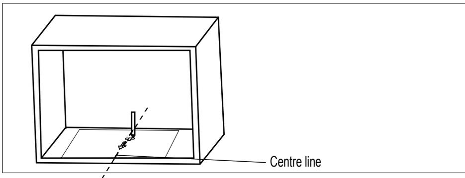
3. Remove the bottom cabinet template and fix the mounting plate with screw A.
