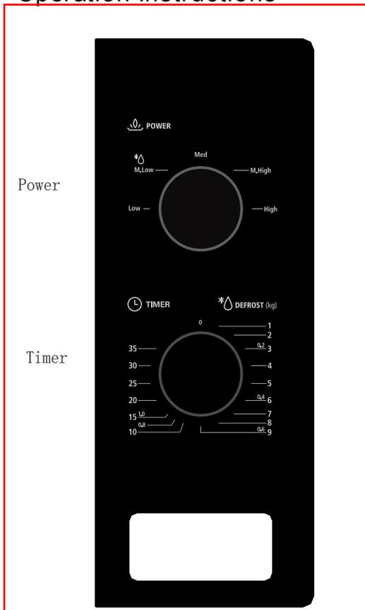
1. To set cooking power by turning the power knob to desired level.
