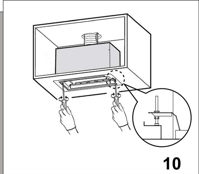
Open the grease filter and remove the two fixing screws with a screwdriver. Lift up until it is fully installed in the bottom of the cabinet. Tighten the screws securing the extractor hood.
