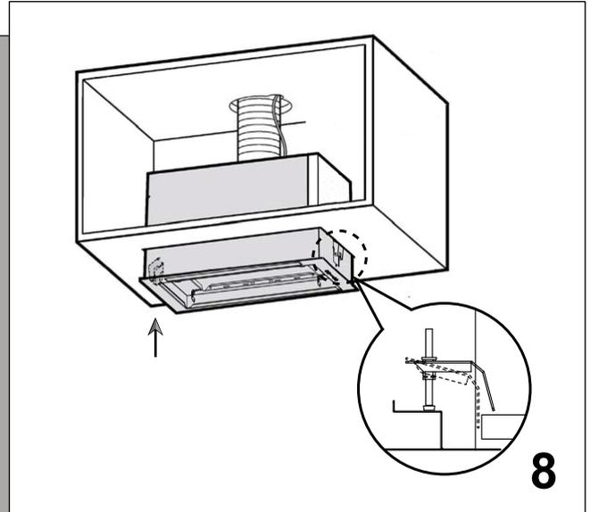
Insert the extractor hood from the bottom up into the cabinet until the locking bracket rests on the bottom shelf.
