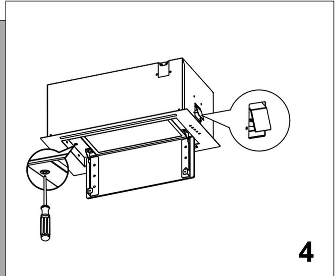
Prior to installation, open the oil baffle and turn the bolt clockwise with a screwdriver to loosen it for easy installation. Loosen the mounting structure tightly fitted to the housing with a screwdriver to facilitate the installation of the entire machine.
