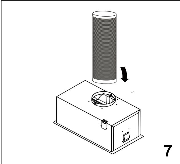
Attach the exhaust pipe to the pipe adapter and place it over the extractor hood as shown.
