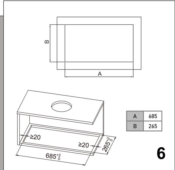
Mark the size of the cut-out according to the dimensions of your bonnet.
