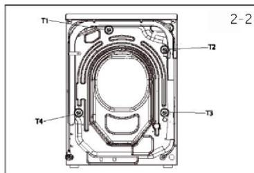
1. Retire os 4 parafusos (T1 - T4) (Fig. 2-3).
