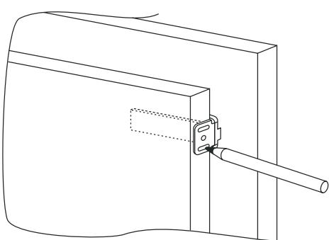
Connect the appliance door to the cabinet panel keeping the loader slots as guidelines.
