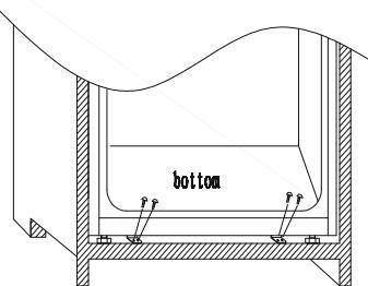
Fit the seal to the appliance, cut off the excessive part if necessary. Fit the bottom parts with plastic covers.
