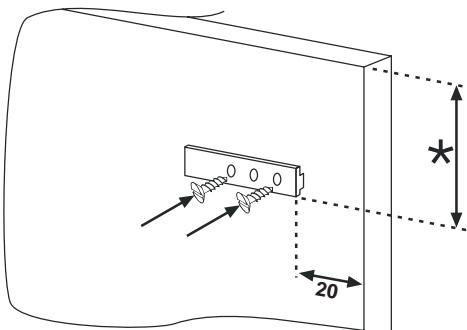
Open the doors of the built-in column and the fridge. Position the built-in loader in the slide, then fit it into the fridge door.
