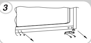
Use the spare hinge and cover from the accessories bag, and fit into the left bottom
