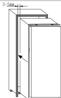
After ensuring the match between appliance door and column door, then screw the appliance upper part to the cabinet
