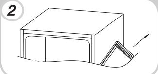
Remove the right bottom hinge and left plastic plugs, and refit them onto the opposite side.
