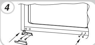
Reassemble the doors and hinges workings from bottom to top, from 1-2.
