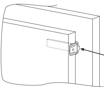
Mark the fixing points for the screws and drill with a bit of a diameter of 2.5mm.
