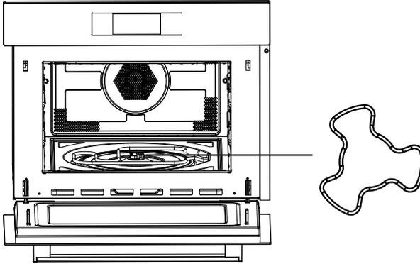
2. Adjust the angle of the tray, the tray roller should point to one of the shaft arm.
