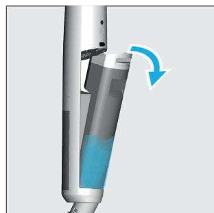
**STEP 2:** Take off the filter and debris collector.
