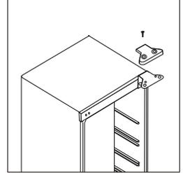
2. Open the door and unscrew the top hinge. Then take the door from the cabinet and place it on a soft pad to avoid damage.
