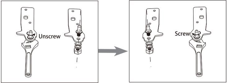
6. Install the hinge at left side and foot base at right side. Then screw two leveling feet with their original parts.
