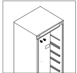
4. Carefully lie down the rear of cabinet on a soft pad. Remove two leveling feet first. Then unscrew the door hinge and left foot base.
