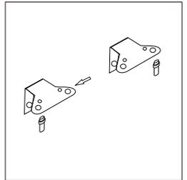
8. Stand up the unit and put the door on the bottom hinge. Make sure the bottom hinge core is inserted in the door hole. Then fit upper hinge with the door. Before tightly fix the upper hinge, try to open the door to check whether the cabinet is sealed well. Finally, screw the hinge cover with hinge.
