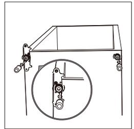
7. Unscrew top hinge pin and mount it to left hole.
