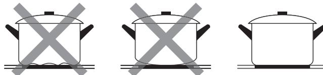
Make sure that the base of your pan is smooth, sits flat against the glass, and is the same size as the cooking zone. Use pans whose diameter is as large as the graphic of the zone selected. Using a pot a slightly wider energy will be used at its maximum efficiency. If you use smaller pot efficiency could be less than expected. Pot less than 140 mm could be undetected by the hob. Always centre your pan on the cooking zone.
