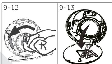
7. Unscrew and remove counter clockwise the pump filter (Fig. 9-12).
