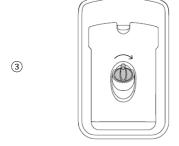
Refit the plug, turning clockwise until secure.
