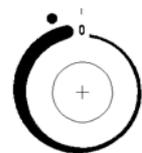
Method B: Select the code switch of corresponding cooking zone, and turn the code switch counterclockwise to adjust the power range from “0” to “15” and the inner and outer rings are heated at the same time. The black dot as shown in the figure indicates that the outer ring is heated at this time.
