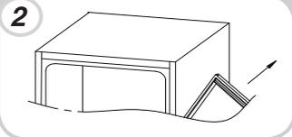
Remove the middle hinge and its connecting pin underneath.
