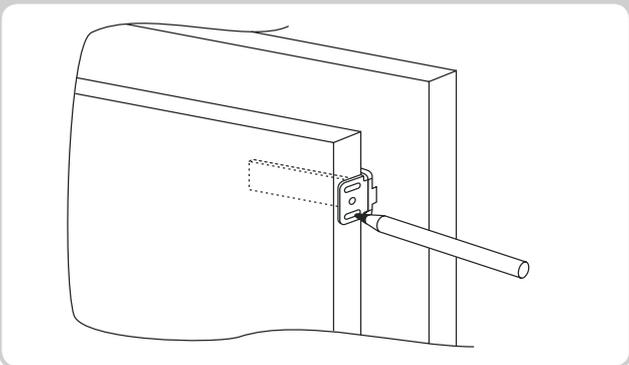
Connect the appliance door to the cabinet panel keeping the loader slots as guidelines.
