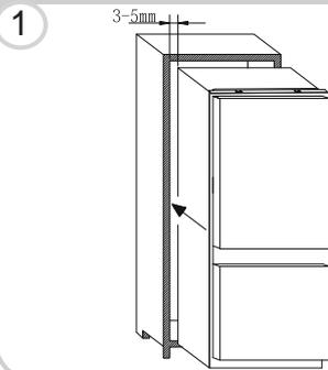
After ensuring the match between appliance door and column door, then screw the appliance upper part to the cabinet
