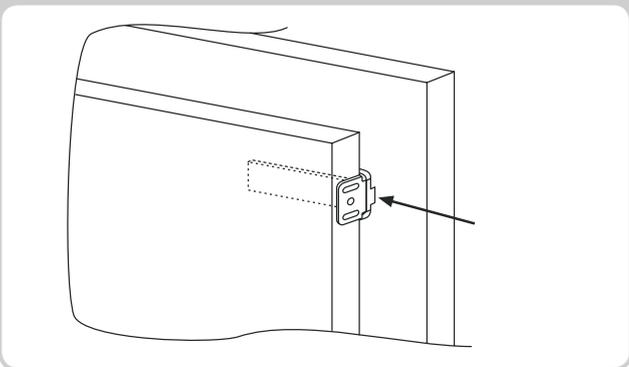
Mark the fixing points for the screws and drill with a bit of a diameter of 2.5mm.
