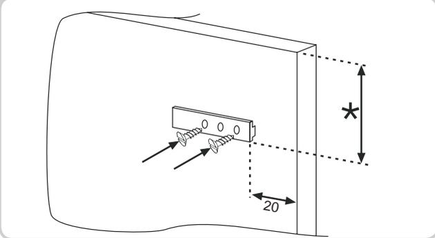
Open the doors of the built-in column and the fridge. Position the built-in loader in the slide, then fit it into the fridge door.
