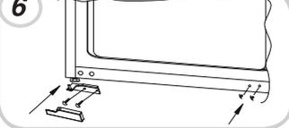
Reassemble the doors and hinges workings from bottom to top, from 1-4.
