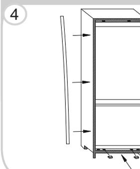
Use a cross-screwdriver to loosen the connecting pin underneath the right middle hinge, and adjust to screw onto the right cabinet wall.
