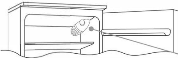
The thermostat box to control the appliance is located inside the fridge compartment on the top right. To check whether the appliance is functioning, make sure that the thermostat knob is not set on "0".
