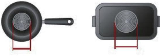
5. If the ferromagnetic part covers only partially the base of the pan, only the ferromagnetic area will heat up, the rest of the base may not heat up a sufficient temperature for cooking.
