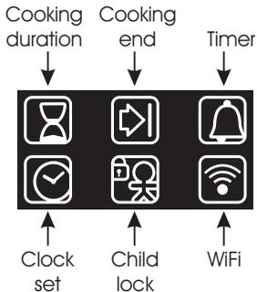
If the oven is switched off, the display shows the clock. When the oven is inactive, all the functions are available except the cooking duration and end of cooking.
