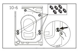
4. Fill the 6 left holes with blanking plugs (Fig. 10-6).
