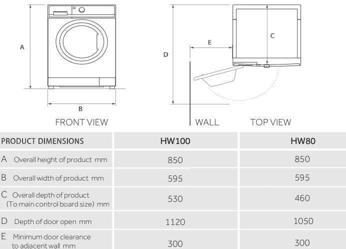
Note: The exact height of your washer is dependent on how far the feet are extended from the base of the machine. The space where you install your washer needs to be at least 40mm wider and 20mm deeper than its dimensions.
