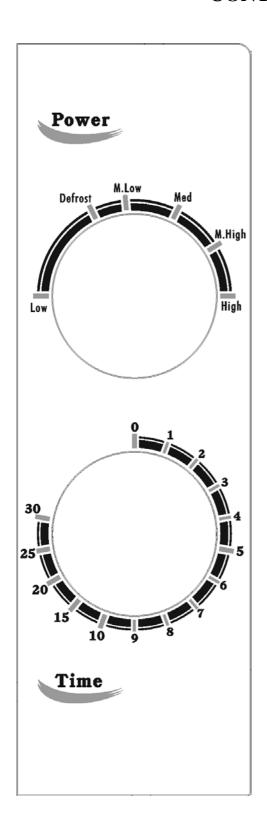
The control panel consists of two function operators. One is a timer knob, and another a power knob.
