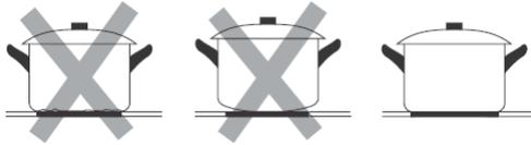
Make sure that the base of your pan is smooth, sits flat against the glass, and is the same size as the cooking zone. Use pans whose diameter is as large as the graphic of the zone selected. Using a pot a slightly wider energy will be used at its maximum efficiency. If you use smaller pot efficiency could be less than expected. Always centre your pan on the cooking zone.
