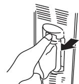
2. Remove collected lint. Place the filter in water and remove lint while wet.
