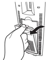
2. Pull the lower end of the lint filter rear cover outward to separate it from the lint filter front cover. Remove lint completely by rinsing with clear water.
