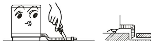
4. If extra drain hose is needed, please make separate purchase. The inner diameter of the extra hose shall not less than 30mm, and the length shall not exceed 1.5m.
