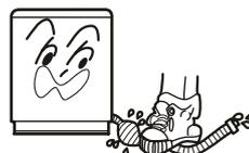
3. If the drain hose is too long, cut it at mid point. To make smooth drainage, cut the front end of the hose slantingly.
