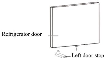
16. Install the Refrigerator compartment door.
