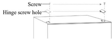
19. Secure the upper hinge to the top left side of the cabinet with the three screws you removed previously. Before you tighten the upper hinge screws, make sure that the top of the door is level with the cabinet and that the rubber gasket makes a good seal.
