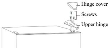
2. Pry the hinge cover up and off, remove the three screws that secure the upper hinge to the door, then remove the hinge.
