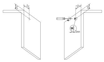
4. Hang the cooker hood on the screws between the two cupboards.
