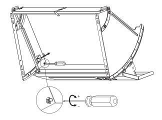
13. Install the adjusting plate, in order to cover the gap between the wall and the bottom of the cooker hood.
