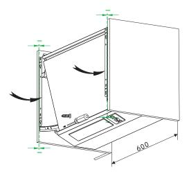
7. Install the outlet as followings: Align the 3 pcs side slots of the outlet with the 3 edges of the blower, insert the 3 edges into the outlet slot, See pic A,then finish as pic B shown.
