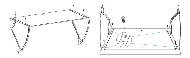
12. The two screws on both sides of the cooker hood can adjust the sliding of the door, according to the weight of the door.
