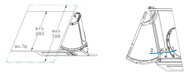
10. Mark the installation position of the door and the size of the fixed screws. If the upper edge of the door is not as high as the upper edge of the cupboards, please adjust the size accordingly. Mark the positions of the screws on the door, and make sure the size is as accurate as 569±1.
