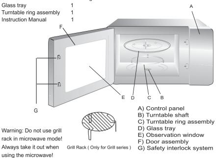
Shut off oven power if the door is opened during operation.
