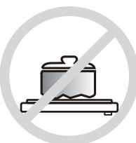
Do not place rough or uneven vessels on the hob, as they may damage the ceramic surface.
