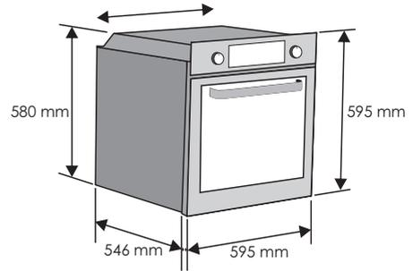
**A GB** If the mounting of the plinth does not allow air circulation, to obtain the maximum performance of the oven it is necessary to create an opening of 500x10mm or the same surface in 5.000 mm<sup>2</sup>
