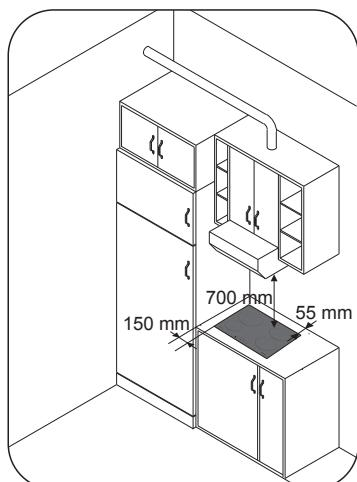
If the bottom part of the hob is adjacent to an area normally accessible for handling or cleaning operations, a separator it must be put 20 mm below the bottom part of the hob.
