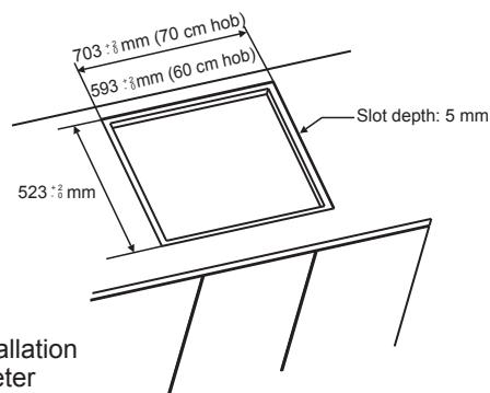
**Note:** Inner perimeter dimensions are same with standard installation
