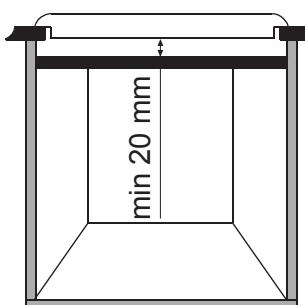
When installing an oven under the hob, separator must not be put and the minimum distance between the bottom part of the hob and the oven must not be lower than 10 mm. Do not install not cooled oven under this hob and install the oven following its own installation requirements.
