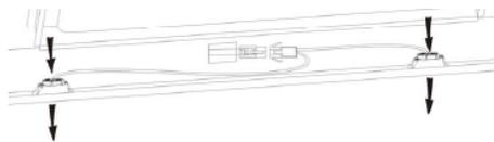
Disconnect the light wiring point and remove the bulb holders and wiring from the hood. Important: It's not possible to replace the bulbs individually, it will be necessary to obtain the bulbs, bulb holders and wiring as a complete part. (LED light: MAX 1.5W)
