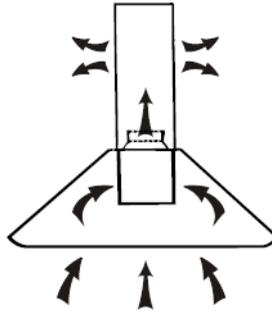
Activated carbon filter can be used to trap odors. In order to install the activated carbon filter, the grease filter should be detached first. Press the lock and pull it downward.
