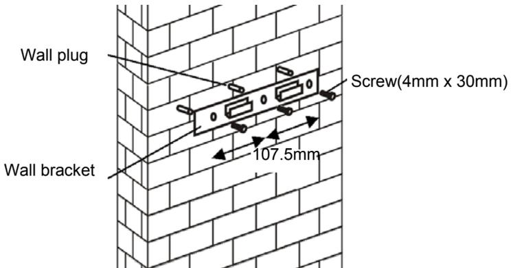
4. Leave up the cooker hood and hang onto the wall bracket hook.
