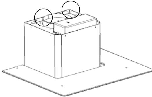
5. Fix the one-way-valve to the air outlet of the cooker hood. Then, attached the exhaust pipe onto the one-way-valve as shown below.
