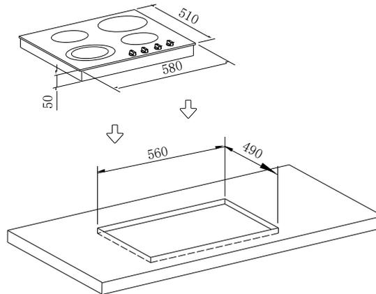
Cut a hole in the worktop that corresponds with the drawing shown above.
