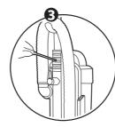
4. Place the crevice tool /dusting brush into the tool holder.
