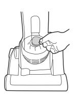
Underneath the dust container you can find the exhaust filter.
