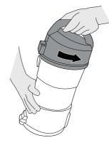
Remove the mesh frame from the filter, then gently tap both filters to release any excess dust.
