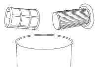
**IMPORTANT!** Ensure the mesh frame is reassembled to the filter before use
