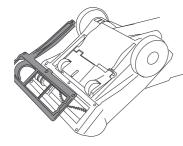
3 Remove brush assembly and check for wear on the belt.
