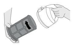
4 Wash both filter and protective mesh under warm water until the water runs clean. Remove excess water by shaking and leave to dry for 24 hours. Reassemble and refit filters to cleaner, only when they are completely dry.
