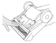
Refit the brush guard with 6 retaining screws.
