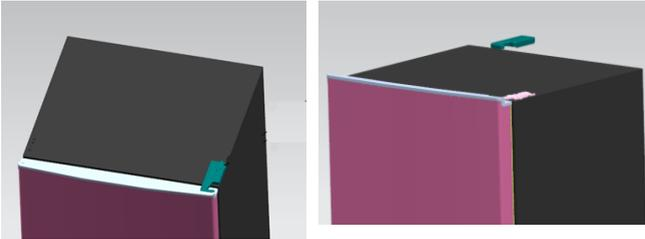
2. Remove the screws fixed the top-hinge with cross-slot screwdriver.
