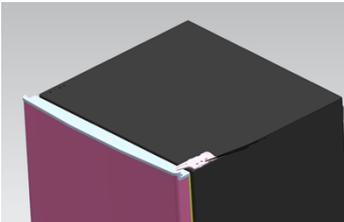
3. Replace the top-hinge and the top-door limit block and the door bearing bush to the other side.
