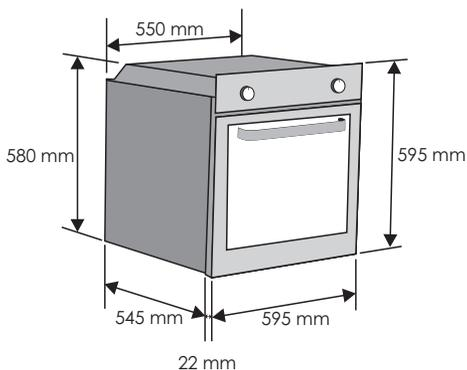
**GB** If the furniture is coverage with a bottom at the back part, provide an opening for the power supply cable.
