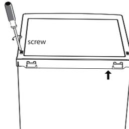
10. With the door closed, check that the door is aligned horizontally and vertically and that the seals are closed on all sides before finally tightening the bottom hinge. Re-adjust the levelling feet as needed.
